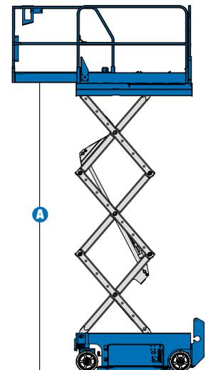
\* The metric equivalent of working height adds 2 m to platform height. U.S. adds 6 ft to platform height.
